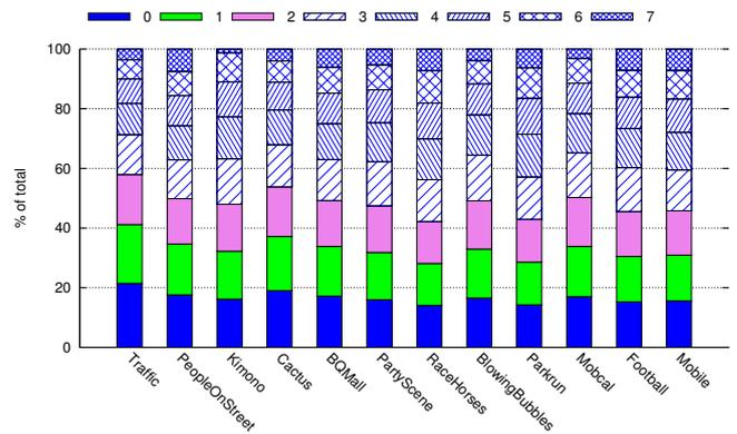
Fig. 1. Write density statistics of each bit in a pixel in reference frame buffer
