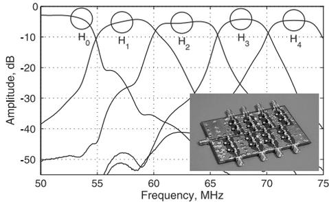
Fig. 3. Channel transfer functions of the employed analog filter bank (five lower channels of the lumped-element inverted cochlea IF channelizer of [10]).
