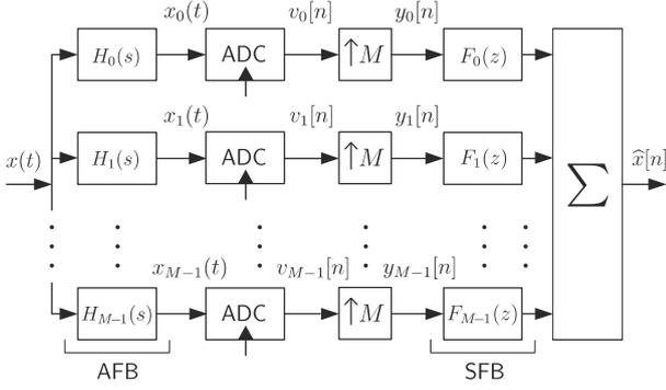
Fig. 1. Conceptual structure of the  $M$ -channel maximally-decimated HFB (“AFB” and “SFB” denote “analysis filter bank” and “synthesis filter bank”).
