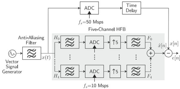
Fig. 2. Schematic of the testing procedure for the real-time signal-reconstruction experiment.
