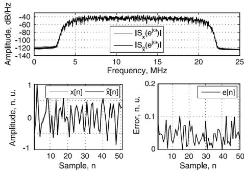
Fig. 6. Frequency and time domain (normalized to  $\max\{|x[n]|\}$ ) responses of the reconstructed ( $\hat{x}[n]$ ) and original ( $x[n]$ ) signals and approximation error for the wide-band signal experiment ( $e[n] = |\hat{x}[n] - x[n]|$ ).
