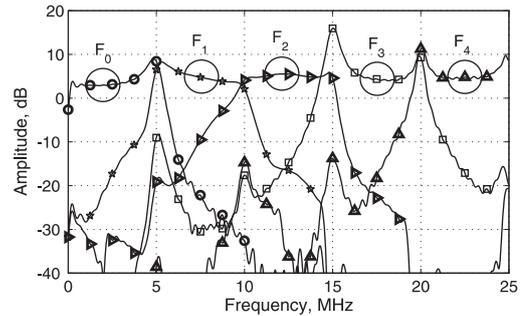
Fig. 4. Frequency response magnitude of the evaluated synthesis digital filters for the wide-band signal experiment ( $L = 200$ ).
